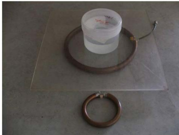
Figure 6. Simple loops used for investigation of inductive compensation of the CSIRO sensor.
