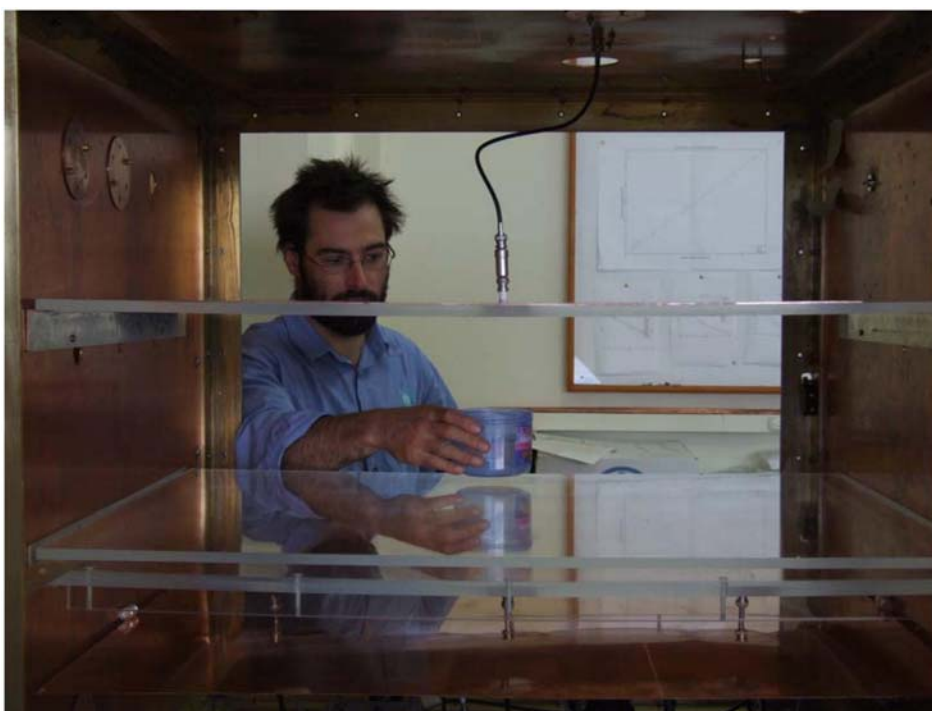
Figure 1. CSIRO laboratory prototype CL sensor configured at CSIRO Lucas Heights Radio frequency laboratory. The view is along the direction the conveyor would normally run in actual applications. Sensor layers are visible towards the top and bottom of the enclosure. A perspex sheet serves to simulate the conveyor.
