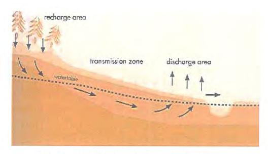
Figure 10. A simple model of water movement in a landscape
