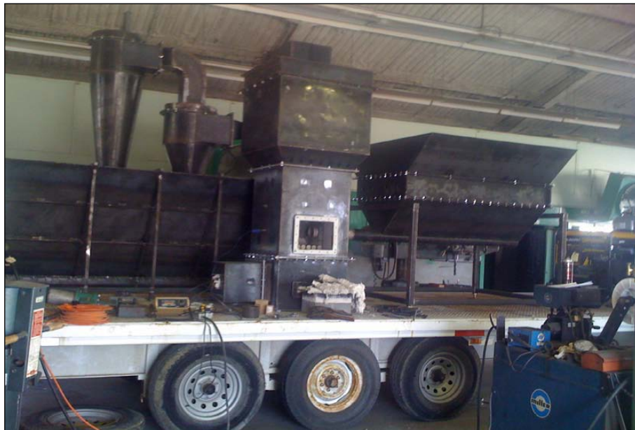
Photograph 11 - TAMU Fluid Bed Gasifier Pilot Plant
