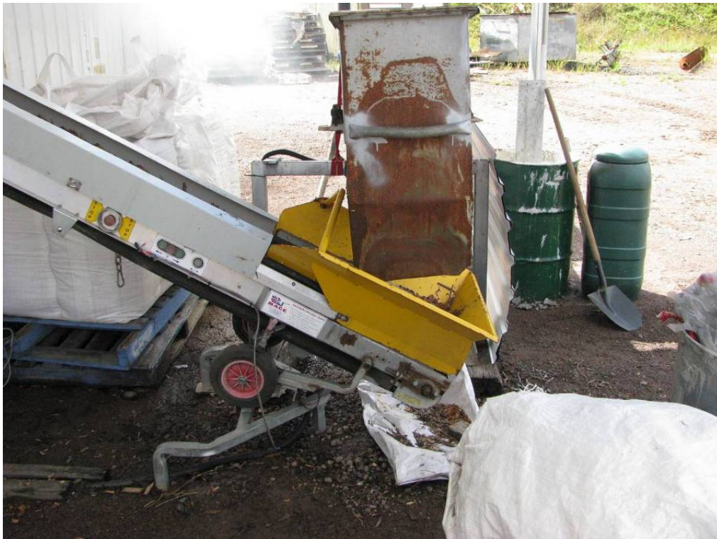
Photograph 20 – Manure feed system into the gasification unit
