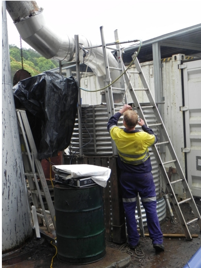
Photograph 44 - Off-gas gas analysis using the Testo 350 analyser
