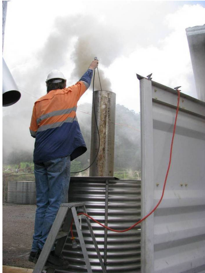
Photograph 22 – Flue gas sampling from the stack
