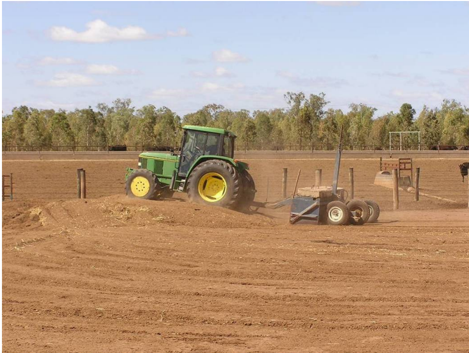
Photograph 2 – Pen cleaning using a box scraper under dry conditions
