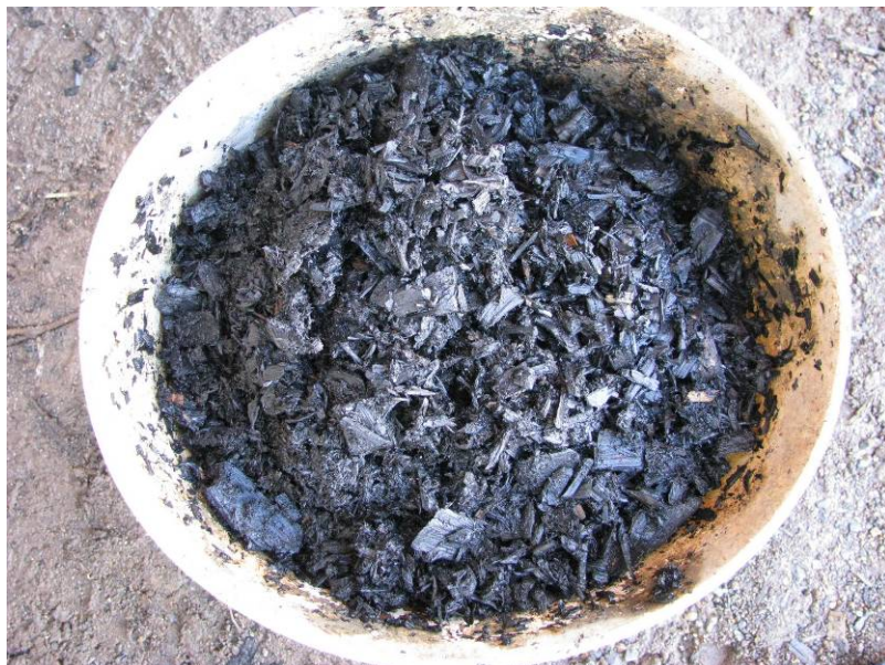
Photograph 23 – Char from the woodchip phase of the gasification
