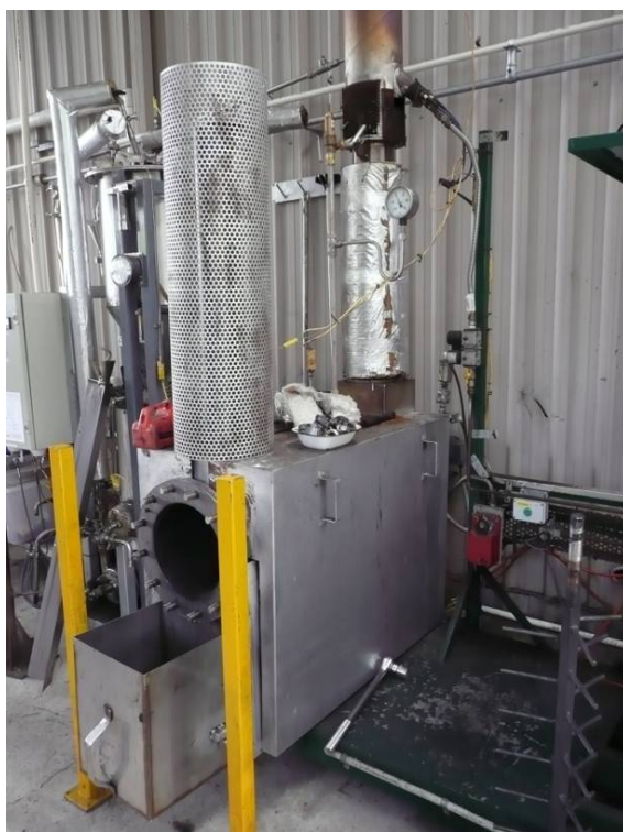
Photograph 38 - PacPyro batch pyrolysis reactor
