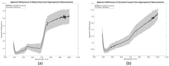
**Fig. 8.** Reflectance spectra of (a) blady grass and (b) serrated tussock computed from 10 samples along the region imaged by SwagBot, showing distinct spectral responses that can be used in identification of different species.
