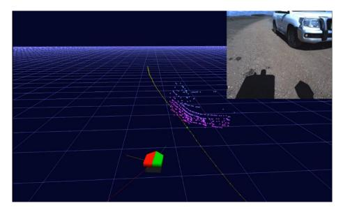
**Fig. 3.** SwagBot obstacle avoidance and local path planning on a farm track at Arthursleigh Farm. The main view is a visualisation of the robot planner and detections of the obstacle (Toyota Landcruiser) from the scanning LIDAR. The inset shows an image from forward-looking camera.
