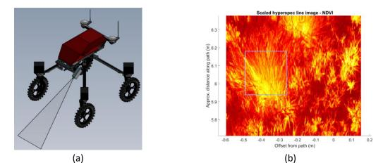
**Fig. 7.** (a) SwagBot with position of Resonon Pika XC2 line scan hyperspectral sensor including the sensor instantaneous field of view projected to the ground plane. (b) Scaled NDVI image generated from SwagBot hyperspectral measurements.
