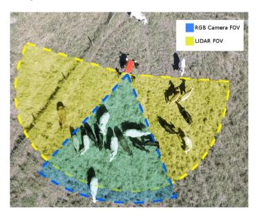
Fig. 9. Colour (RGB) camera and LIDAR sensor fields of view
