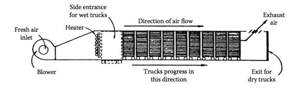
Fig. 5: Tunnel dryer (Mujumdar, 2015)
