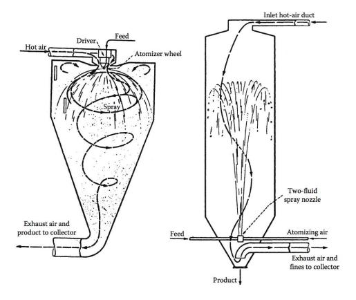
Fig. 8: Spray dryer: drying chamber (left) and cyclone (right) (Mujumdar, 2015)
