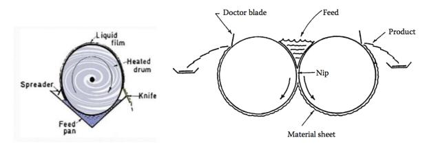
Fig. 6 and 7: Single (left) and double (right) drum dryers (Mujumdar, 2015)
