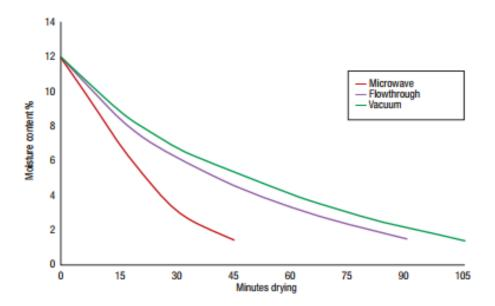
Fig. 14: Moisture content vs minutes drying for different processes (Parikh, 2015)
