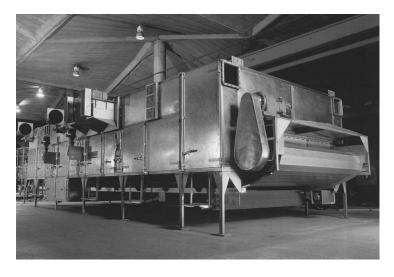
Fig. 13: An image of a thin-film belt dryer (Mujumdar, 2015)
