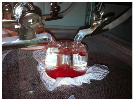
**Figure 6.** A membrane feeder used in BF culture. Blood is provided *ad lib* at the top of the cage with blood heated to 37°C by water recirculated from a water bath. Flies feed through the silicone-nylon membrane attached at the bottom of the feeder.
