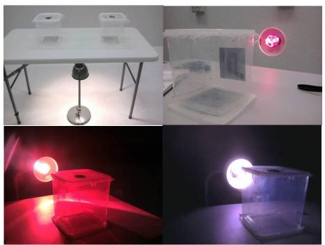
**Figure 12.** Some of the light configurations tested: a) light beneath the table; b) silhouette and light to the side; c) infrared lamp; d) moonlight
