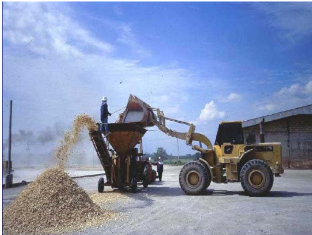
Figure 13. In Thailand, cassava roots are chipped and sun-dried on large concrete drying floors. Photo source: Howeler (2009).
