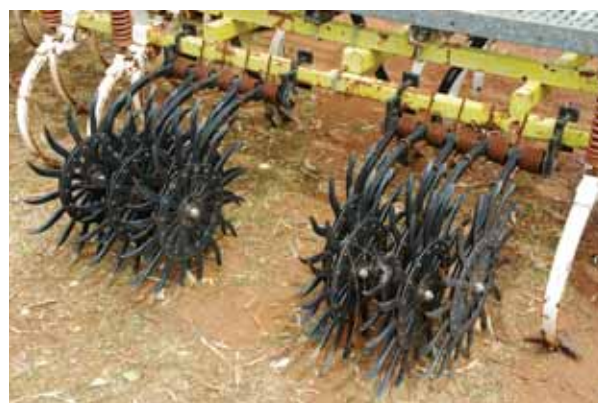
Yetter wheels over the rows break any surface crust and knock out weeds without greatly disturbing leucaena seedlings.
