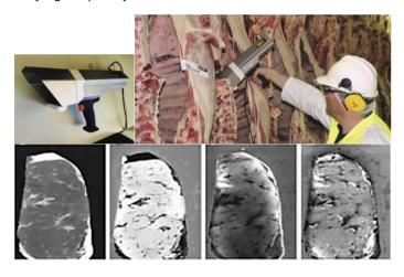
MLA has put many carcase measurement technologies through their paces, but SEXA, DEXA, CT scanning, 3D camera, and near-infrared spectroscopy, show the most promise as reliable and cost-effective tools which suit the red meat processing industry.
