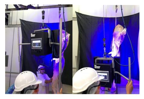
Figure 4. Scanning of a beef carcase using the Hot Spot Camera Scanner.
