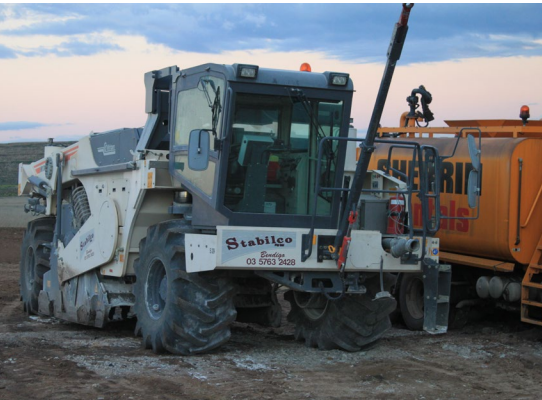
Large reclaimer/stabiliser for mixing binder agent into base material
