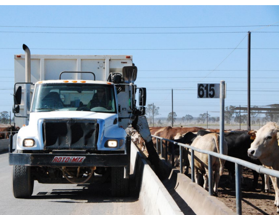
Feed delivery trucks usually feed out on the same side as the driver with left or right hand drive.
