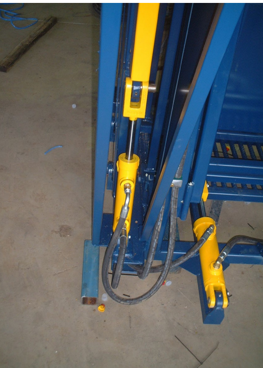
Power-assisted hydraulic gate
