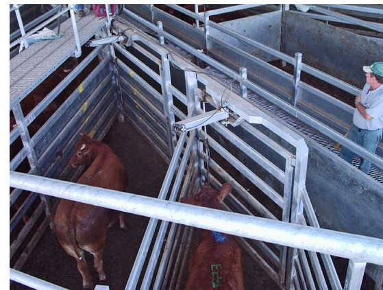
Pneumatically-swing gates used in stacking pens.
