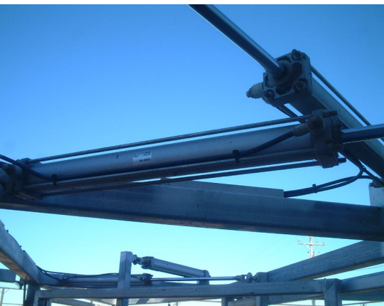
Power-assisted pneumatic gate
