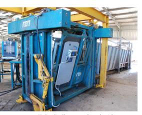
Hydraulically-operated crush with multiple features.
