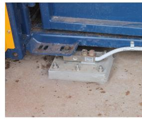
Crush mounted on load cells for weighing.
