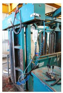
Hydraulic controls for a crush.
