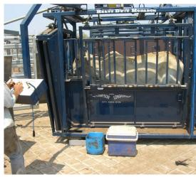
Full-length squeeze where animal can stand freely without being head bailed, but this does not provide safe access to the head.
