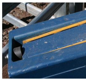
Wear pads reduce wear, and rubber stoppers reduce noise, shock and fatique.
