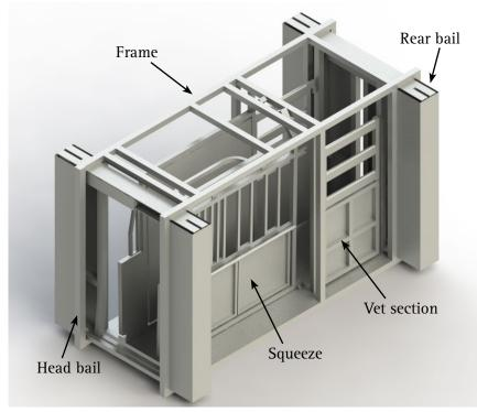
Figure 2. Features of a crush
