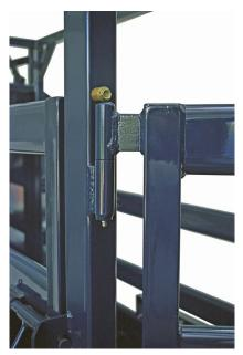
Grease nipples on hinges for easy movement.
