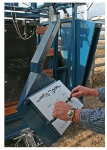
Operating console for a pneumaticallyoperated crush.
