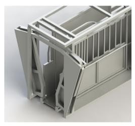
Figure 3. Schematic example of straight bar V-opening crush
