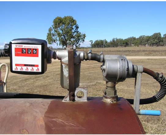
Fuel hose in good condition, with fuel filter and meter to record fuel usage.
