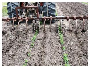
Yetter wheels over the rows break any surface crust and knock out small weeds without greatly disturbing leucaena seedlings.
