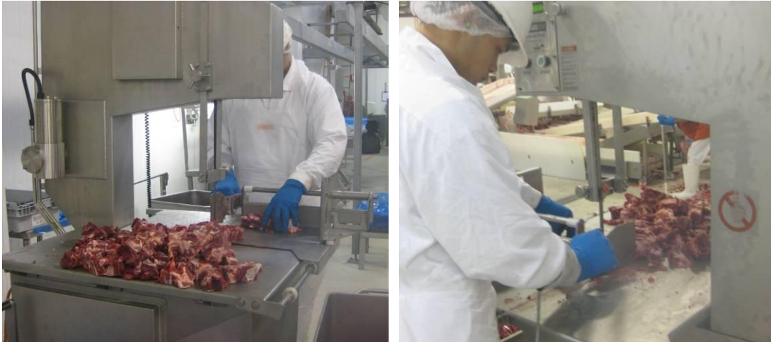
Fig.12 Bladestop installed at ACC
