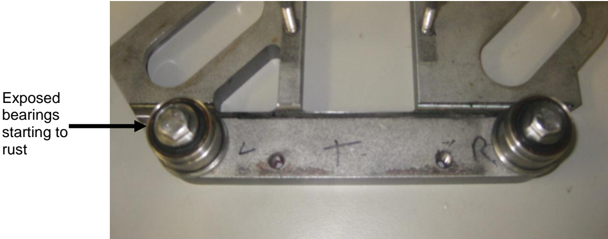
Fig.16 Previous Bearing Sleeve Design
