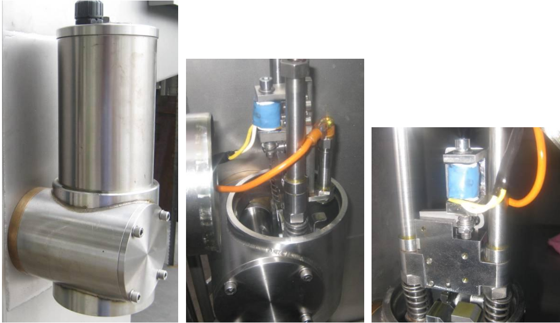
Fig. 8 Views of the inside and outside of the new back half of the Bladestop mechanism on the ACC Saw
