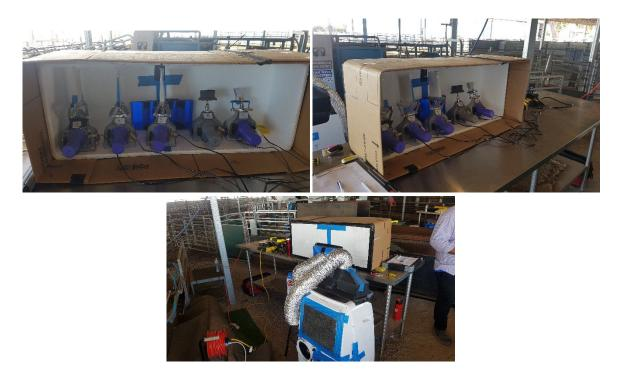
Figure 11 Portable cooling system made for Live sheep measurement at Katanning Research Facilities.
