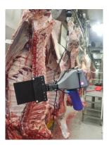
Figure 7 Beef carcase hot P8 and Rib fat depth measurement at abattoir kill floor using a spring balancer.
