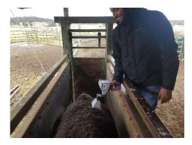
Figure 10 Live cattle measurement at feedlots using Horn Antenna with new antenna holder.
