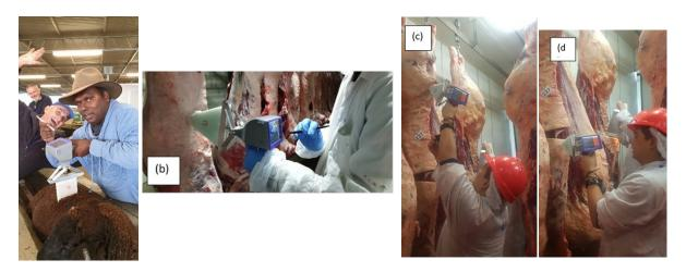
Figure 6 The proposed Microwave System used for various measurement (a) Live sheep measurement at feedlots (b) Lamb carcase measurement at abattoir (c) Beef carcase P8 fat depth measurement at abattoir (d) Beef carcase Rib fat depth measurement at abattoir
