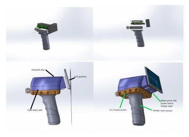
Figure 12 Proposed new design for Microwave handheld unit.
