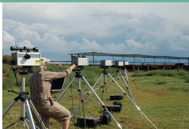
Measuring emissions from a feedlot using open-path lasers.
