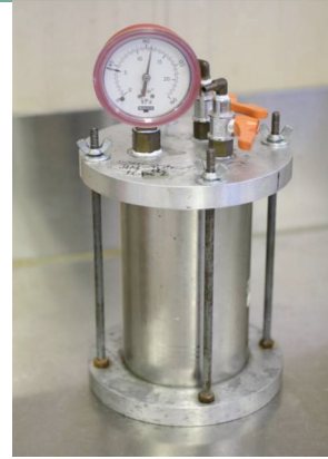
Anaerobic canister for maintaining Hydrogen-rich growing conditions.
