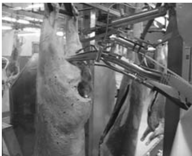
Three robotic systems to alleviate worker strain and injury were installed in Peel Valley, a sheep processor in Tamworth, NSW.
