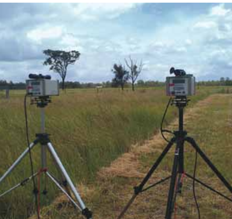
Above: CSIRO's Dr Chris McSweeney with Brahman cattle grazing leucaena at the Brian Pastures Research Station in Queensland. Below: Equipment used to measure methane emissions. Images courtesy of CSIRO.
