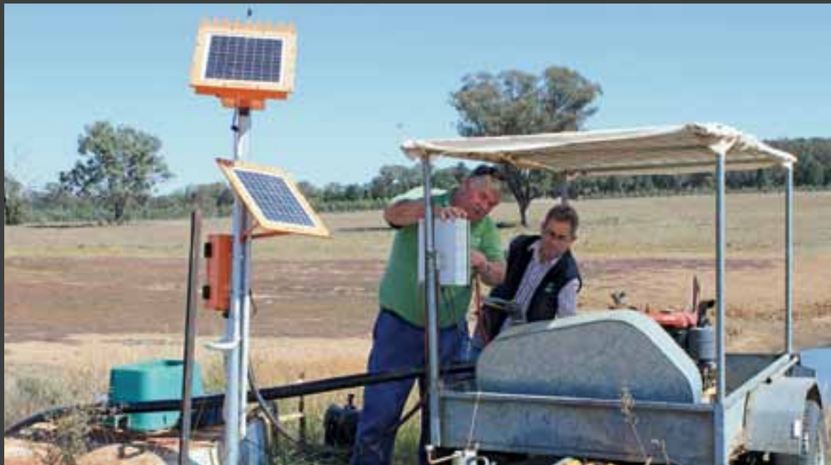
Left: The portable telemetry equipment can follow the mobile pump unit to additional sites, providing additional value for the capital outlay and creating flexibility.
