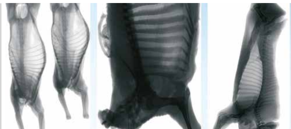
DEXA technology provides timely, accurate and objective information on the lean meat, bone and fat composition of each carcass.
