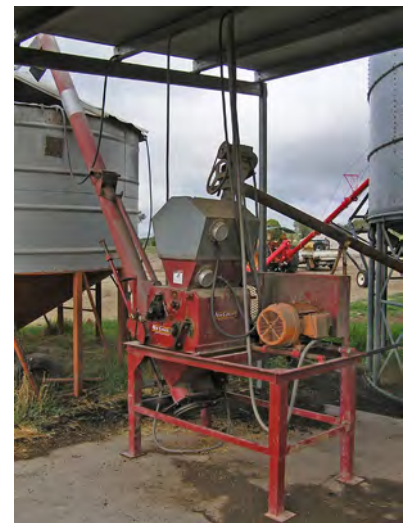
A single electric belt-drive roller mill. Grain is conveyed to the hopper above the rollers and then to a holding bin.
