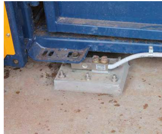
Crush mounted on load cells for weighing.
