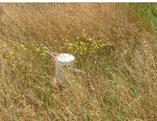
Maintenance of site – grass and weed seeds blocking the funnel of the rain gauge will affect data quality.
