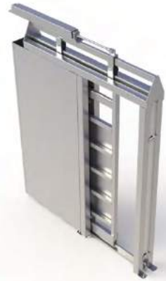
Figure 7. 3-D graphic of a slide gate
