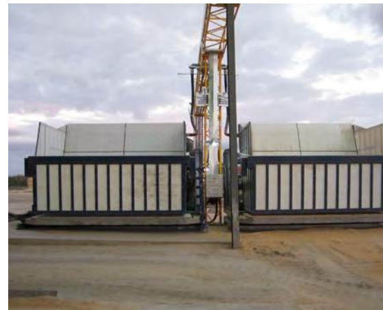
This dual batch-box system is located externally to the commodity storage. No liquid feedstuffs are added at this point.
