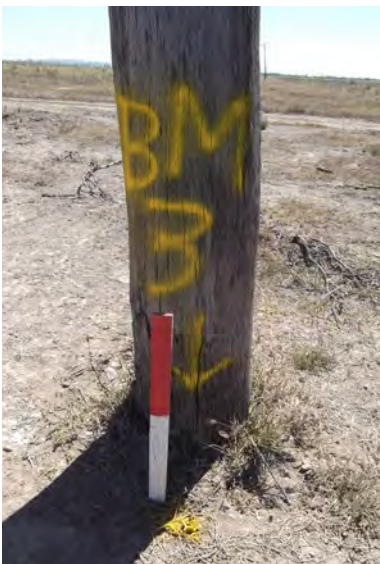
A poorly located Temporary Bench Mark (TBM) sited near to infrastructure not affected by earthworks.
