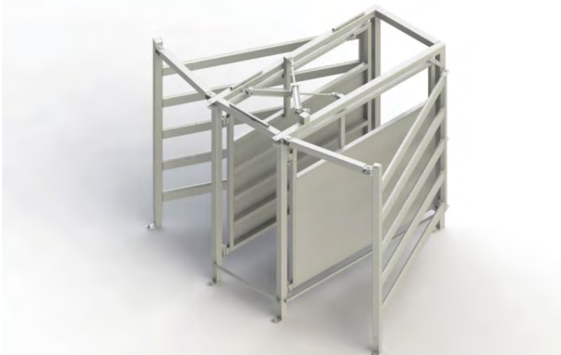
Figure 8. 3-D graphic of a 3-way draft
