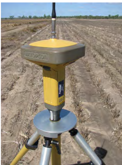
RTK-GPS is commonly used survey equipment.
