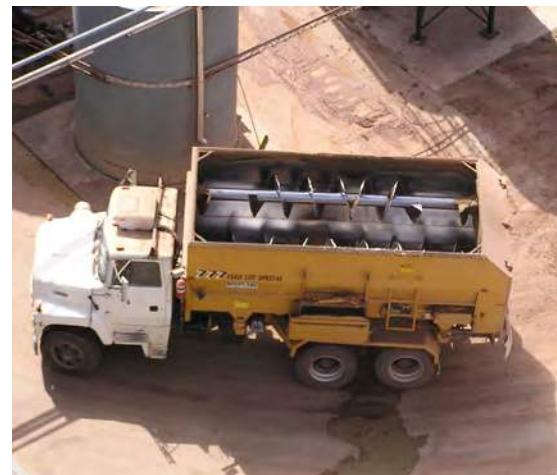
Horizontal screw mixing augers in the feed truck.
