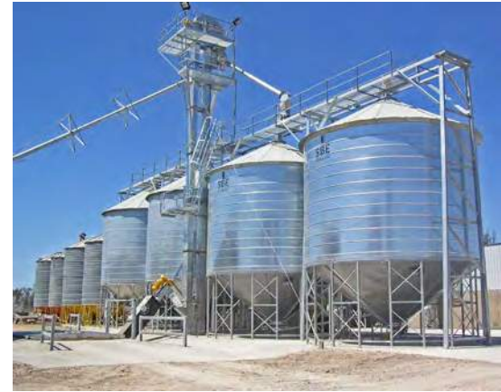
Receival grid, grain handling and cone-bottom silos. The grain is conveyed from the receival grid to a bucket elevator, with gravity fall to a horizontal conveyor for transport to the silo of choice. The height of the bucket elevator is reduced by using a horizontal silo loading conveyor.
