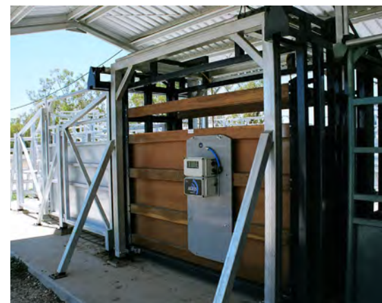
Suspended weigh box and NLIS race reader.
