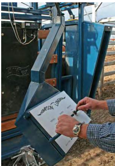
Operating console for a pneumatically-operated crush.
