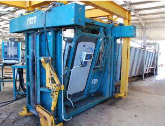
Hydraulically-operated crush with multiple features.
