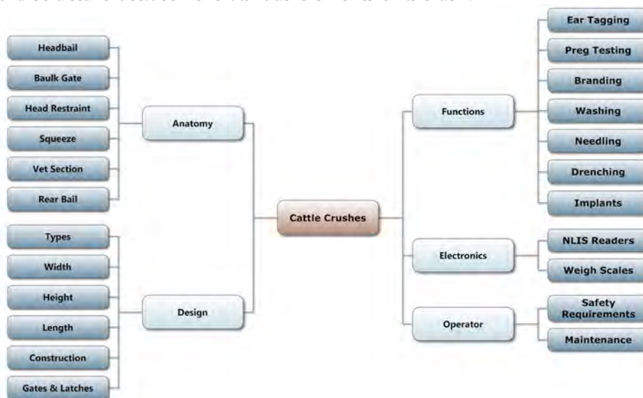
Figure 1. Conceptual representation of crush design factors.
