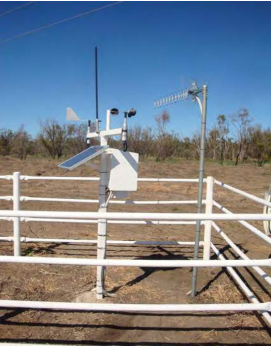
Typical 2 m solar-powered AWS with remote access.
