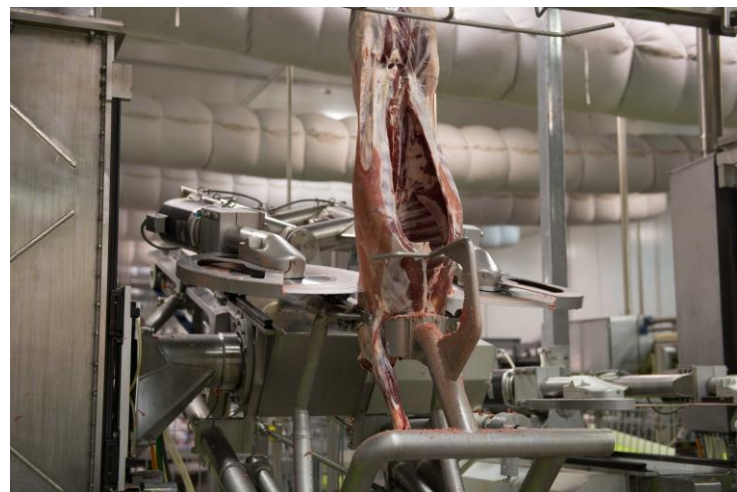
Figure 1. LEAP III lamb processing automation
