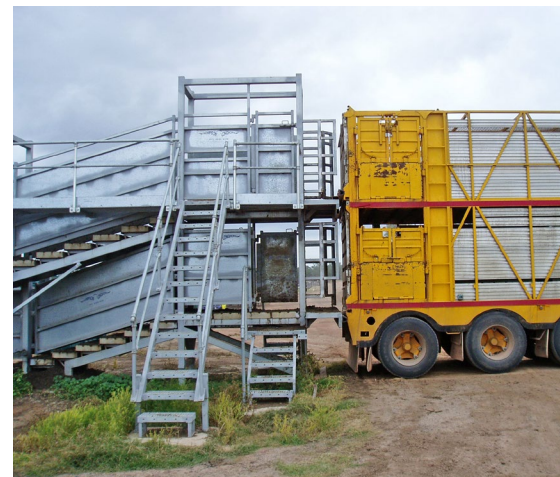
Double deck steel ramp for loading livestock transport vehicle. The front of the ramp has batwing gates and a short platform.
