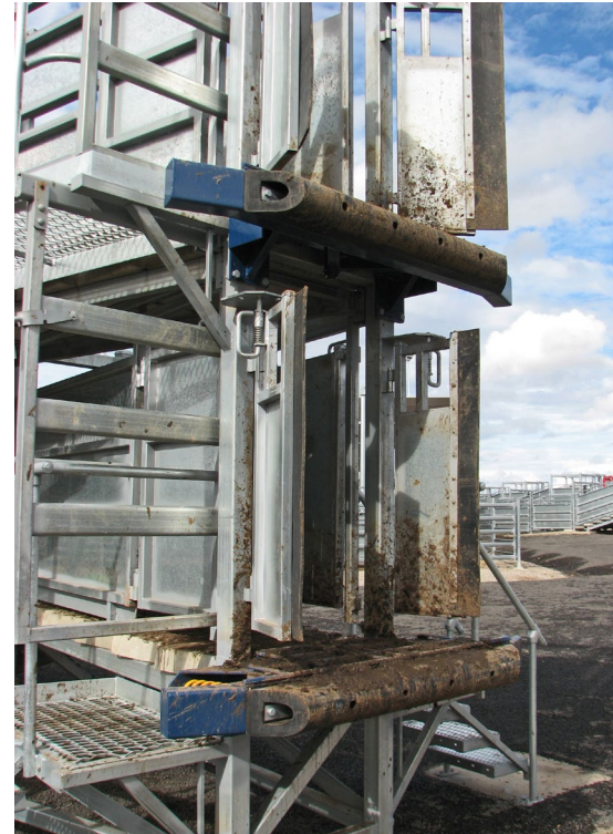
D-mould rubber front for cushioning impact, and slide gates behind the batwing gates.
