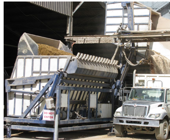
A dual batch-box system installed at the end of the commodity storage. The loader can continue to load one batch box while the other is tipped into the feed truck. The front of the batch-box holds liquid dispensing equipment.
