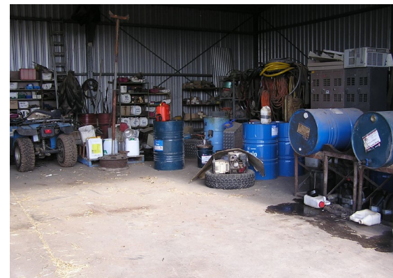
Clear area for small vehicle repairs, but poor type of drip trays under the oil drums.
