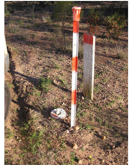
Permanent survey mark (PSM) and marker post.
