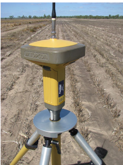
RTK-GPS is commonly used survey equipment.
