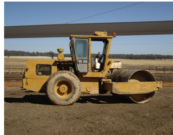
Smooth-drum rollers are used to compact the high spots until the surface is smooth—usually after a grader has levelled the surface.
