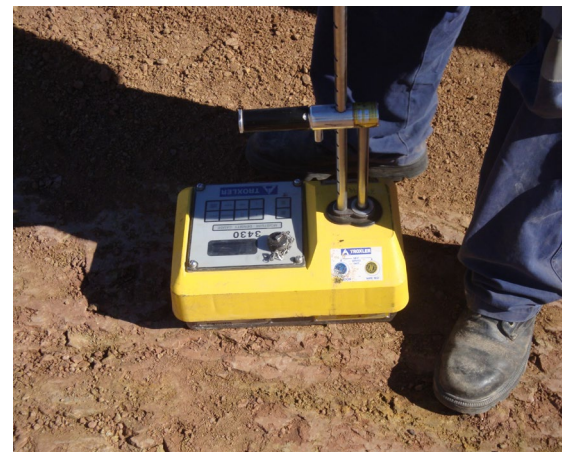
Field testing soil compaction
