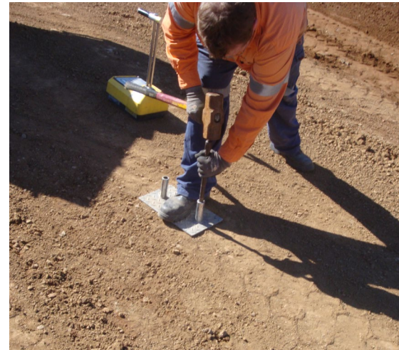
Field testing soil strength
