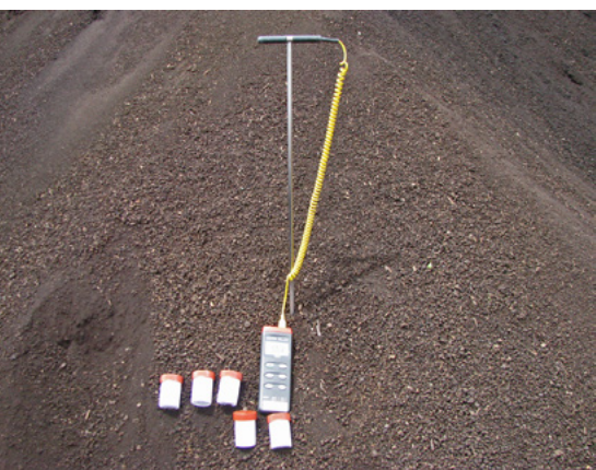
A probe can be used to measure temperature in the compost windrow.
