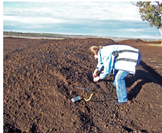
Temperatures and moisture content are checked in windrows to monitor the process.
