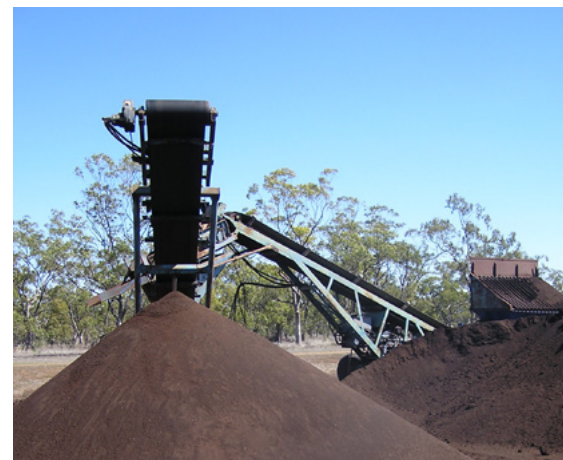
Screening converts lumpy compost into a loose, friable product that can be spread more evenly.
