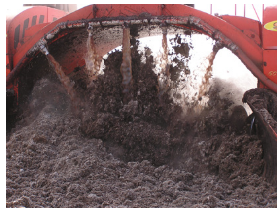
Effluent being applied by self-propelled windrow turner to raise moisture content
