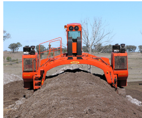
Compost is turned after at least three days at high temperature.
