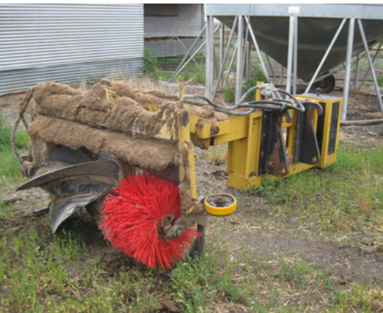
Rotating brush cleaners can be used for feedbunk cleaning.
