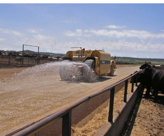
A water cart can be used to suppress road dust.
