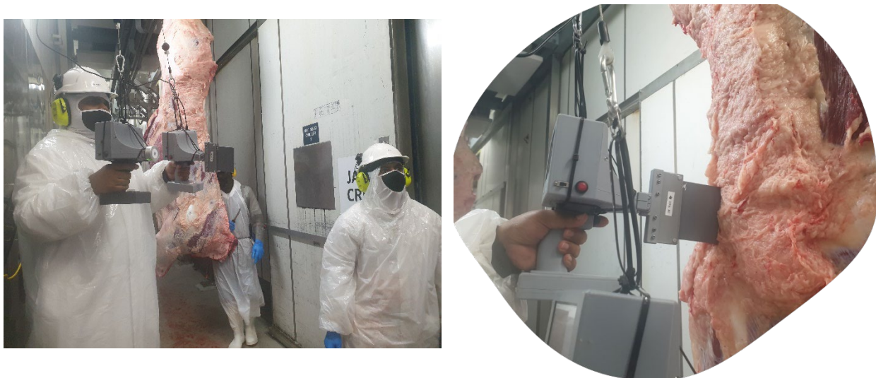
Figure 4: Microwave scanning of hot carcass rib fat site on the chain
