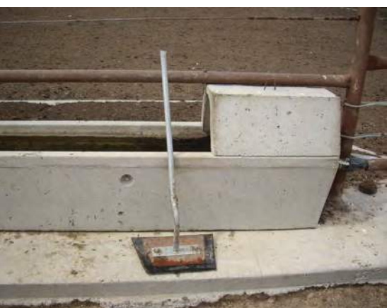
Concrete float cover and a trough cleaning device shaped to exactly fit the trough's internal shape.
