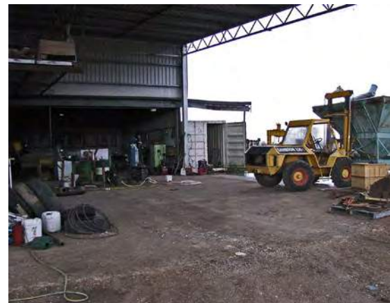
A large machinery workshop with an open side offering good access, good ventilation and natural lighting – but little protection from the weather.
