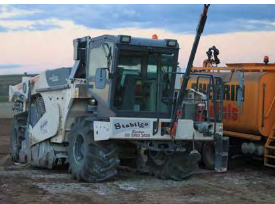
Large reclaimers/stabilisers for mixing binder agent into base material
