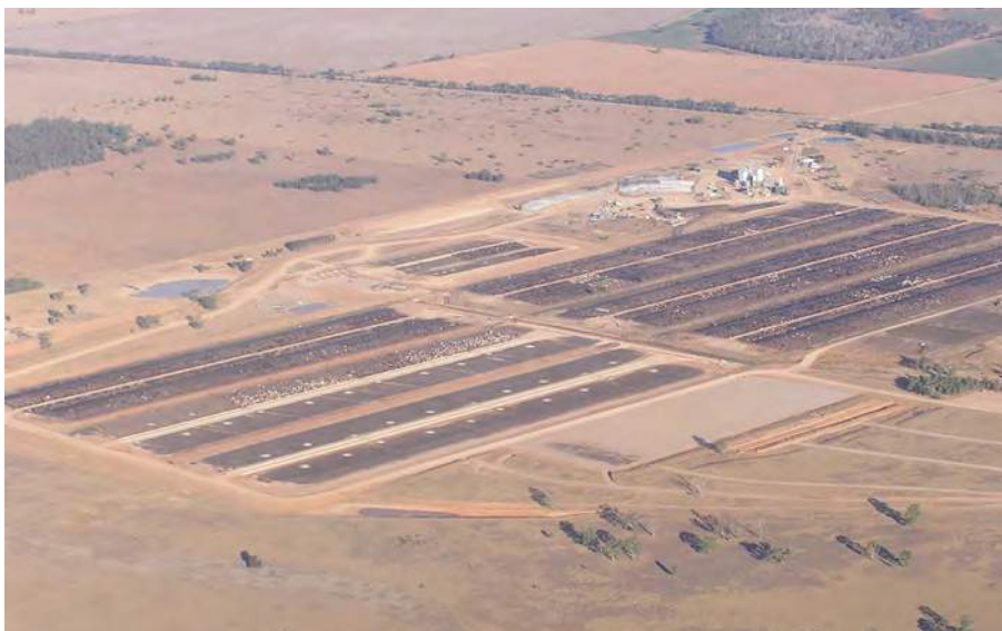
Back-to-back straight rows with feed processing and cattle handling located on one side.
