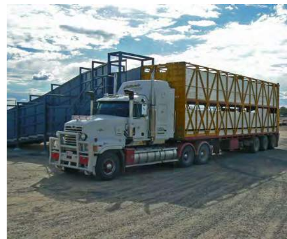
Double deck ramp – side loading of livestock transport vehicle
