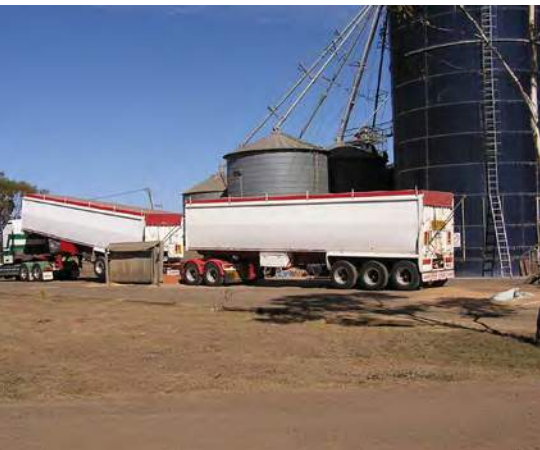
A permanently situated, drive-over grain receival hopper for fast unloading of trucks.
