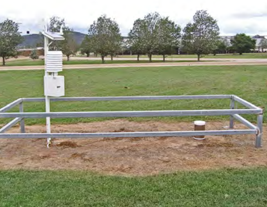
Well-sited 2 metre AWS with no nearby obstructions and a low security fence.
