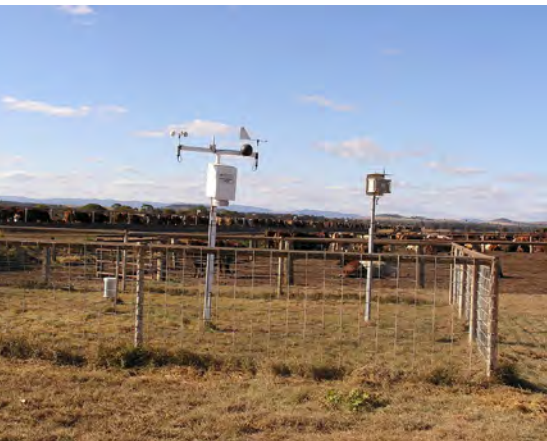
Well sited 2 metre AWS located in the centre of a feedlot with no nearby obstructions and a security fence to keep out livestock.
