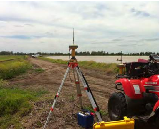
RTK-GPS survey base station and rover mounted on ATV
