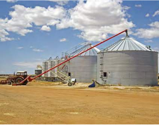
A tractor powered auger used for loading these flat-bottom silos. Note the PTO-powered auger at the base of the silo for unloading grain from the silo.
