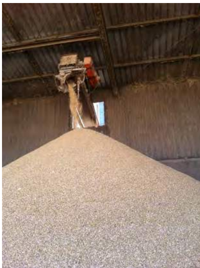
Locating the commodity storage facility adjacent to the feed mill allows processed grain to be discharged directly into a storage bay.
