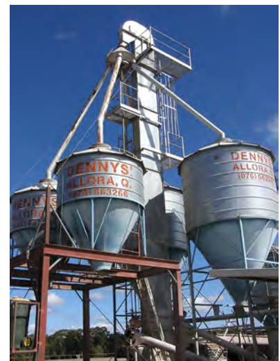
Bucket elevator, diverter and cone-bottom silos. The feed delivery vehicle is loaded directly from the elevated silos.
