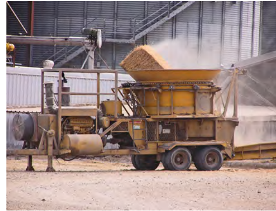
Diesel powered portable tub grinder. This model incorporates a dedicated power plant, but tractor-driven PTO systems are also available.
