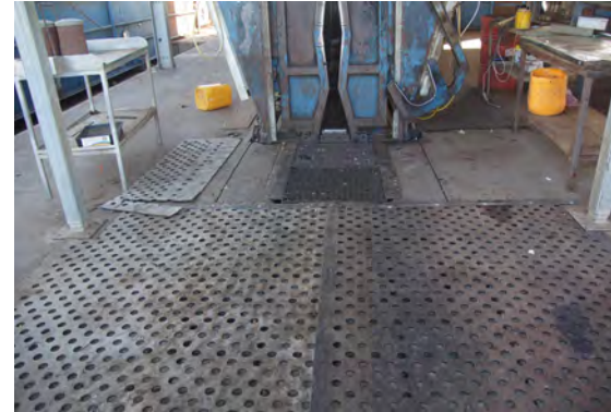
Rubber belt soft flooring with 40 mm holes punched in the rubber for non-slip effect.
