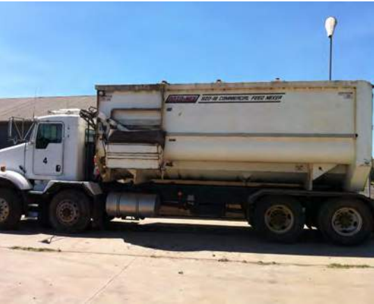
Selection of make and model of commercial feed delivery trucks is driven by personal experience and the size of the feedlot. This imported left hand drive truck delivers feed to the left.
