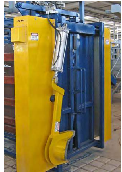
Pneumatic head restraint and pneumatic chin lifter. Yellow panels highlight nip/crush points and moving parts to handlers.
