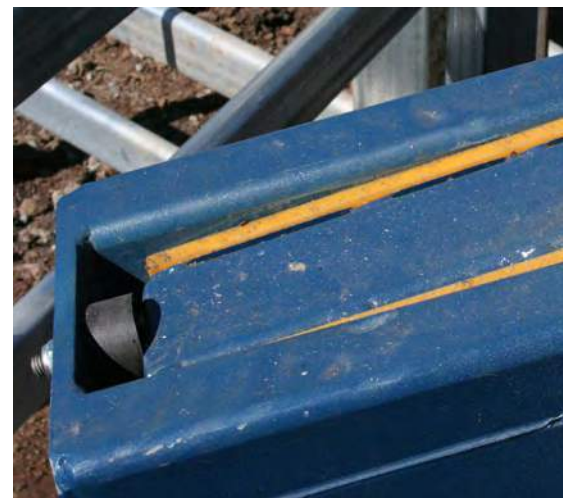
Wear pads reduce wear, and rubber stoppers reduce noise, shock and fatigue.
