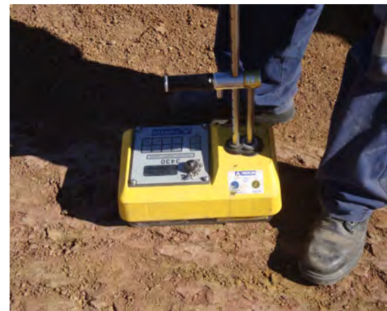
Field testing soil compaction
