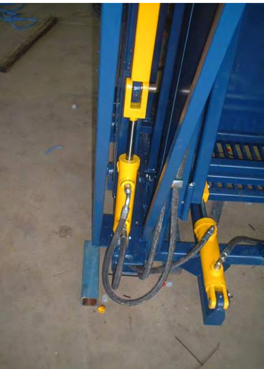
Power-assisted hydraulic gate
