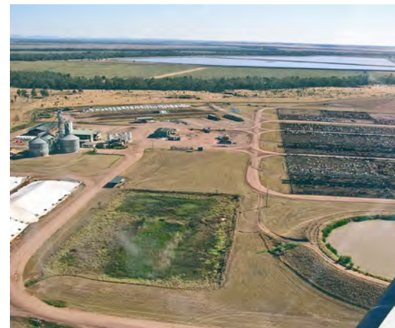
Grain handling and storage facilities need all-weather access, and should not interfere with operational traffic to pens.
