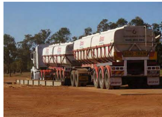
A level concrete pad at the approach to a weighbridge keeps trailers level if prime-mover and trailers are weighed separately.
