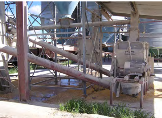
Two single roller mills paired to increase capacity, or to mill two different grains at the same time.
