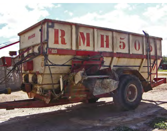
This 5.5 tonne tractor drawn horizontal mixer requires 95–105kw at the PTO.
