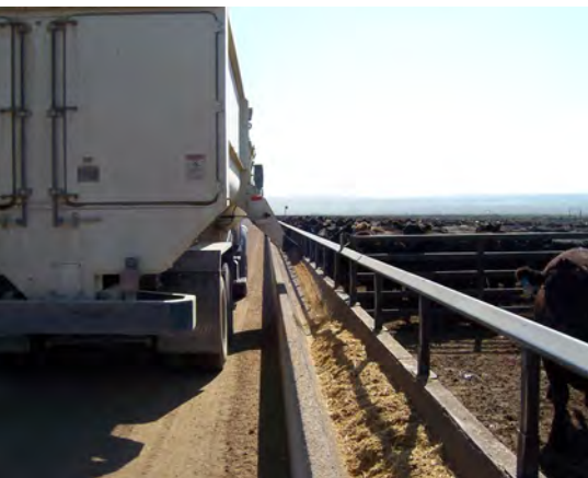
A feed-out chute on the same side as the vehicle operator minimises spillage and wastage when dispensing feed (i.e. right hand drive vehicle with right hand side delivery chute). A rubber extension on this chute minimises damage from impact with the feed bunk.
