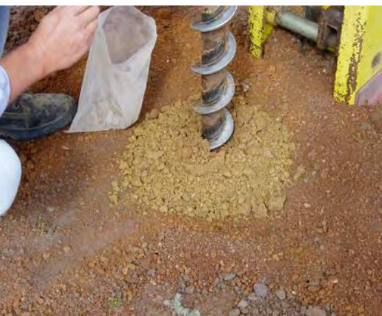
The soil sample should be taken straight off the auger and its depth recorded.
