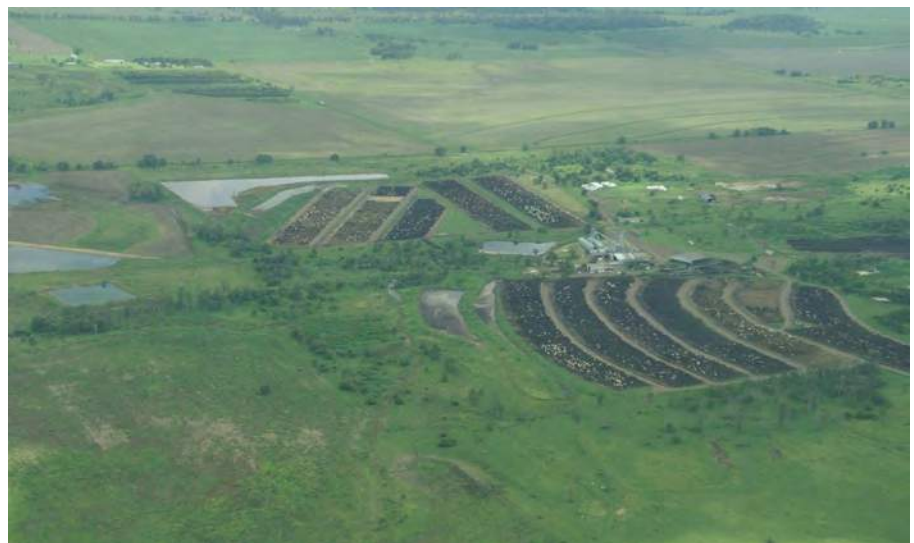
Sawtooth pen layout around the hill with central feed processing area. A curved layout is not desirable.
