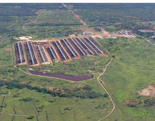
This holding pond is designed to fit the topography between the feedlot pens and a local drainage line.
