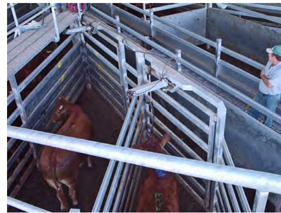
Pneumatically-swing gates used in stacking pens.
