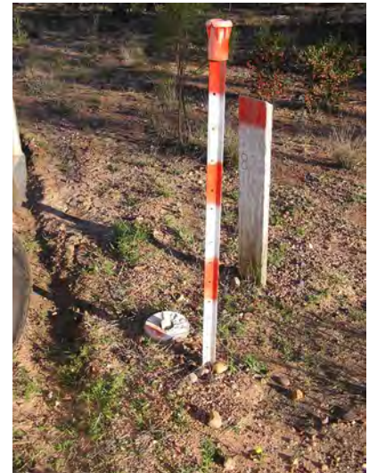
Permanent survey mark (PSM) and marker post.
