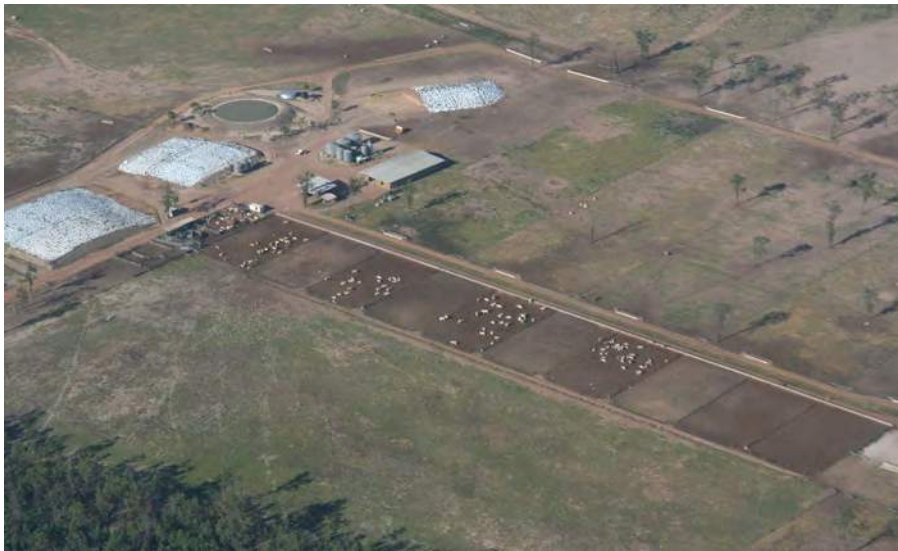
Small feedlot with single row of equal-sized pens. This layout has sufficient area for expansion.
