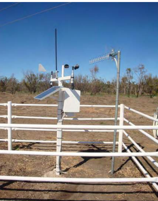
Typical 2 m solar-powered AWS with remote access.
