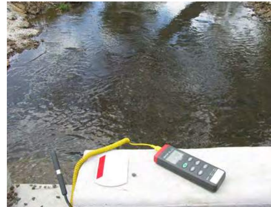
Only pH and EC water quality parameters may normally be assessed in-situ. All other parameters must be tested at a NATA-accredited laboratory.
