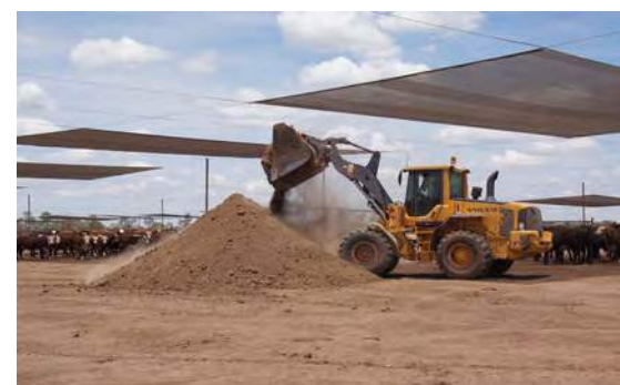
Shade structures should be high enough for machinery. Higher shade structures offer better ventilation but limit the area of shaded footprint and have higher wind loading.
