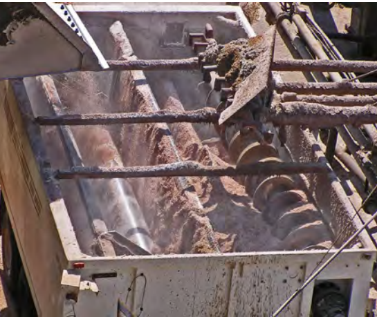
Paddle type mixer in the feed truck. The paddles can be seen under the loader bucket. Liquid supplement nozzles are under a shield.
