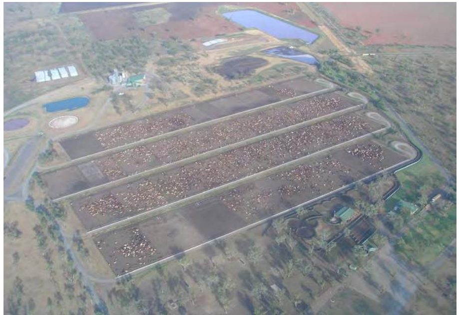
Medium-sized feedlot with sawtooth pen layout and straight rows. The cattle handling system is at the bottom of the site while the feed processing system is on the opposite side of the feedlot.
