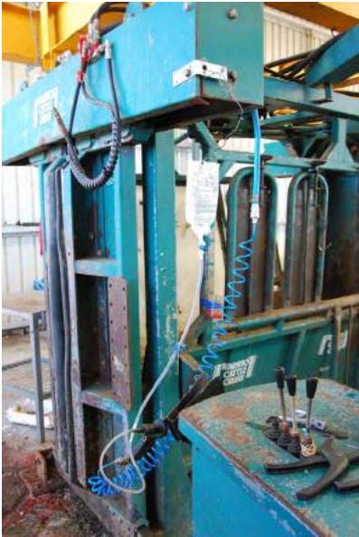
Hydraulic controls for a crush.
