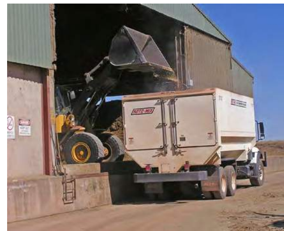
Typical bunker feed delivery system. The loader transfers ingredients to a truck mounted mixer, which then mixes on the go during delivery to the pens. Liquid supplements are loaded at a separate location.
