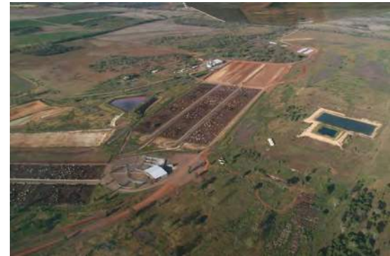
The siting of this holding pond allows for expansion and its geometry suits the topography of site.
