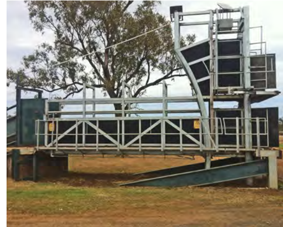
Adjustable steel ramp for access to double deck livestock vehicles. Note the adjustable batwing gates on the top deck platform.
