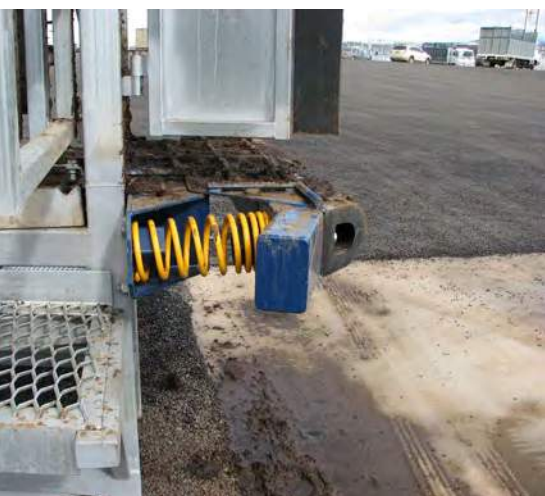
Spring-loaded front with D-mould rubber for cushioning impact.
