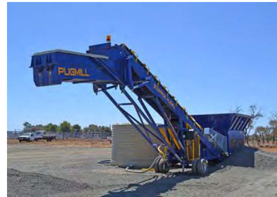
A pug mill machine is a continuous mixer commonly used for obtaining a dense, well-graded, uniformly mixed material.
