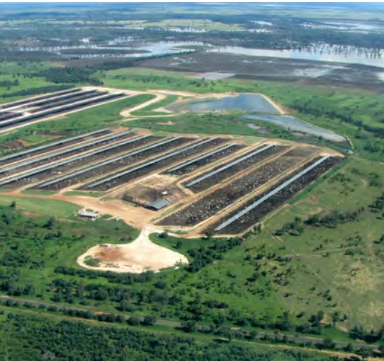
Feedlots should be sited outside of the 1 in 100 year flood coverage area and have road access during major flooding.
