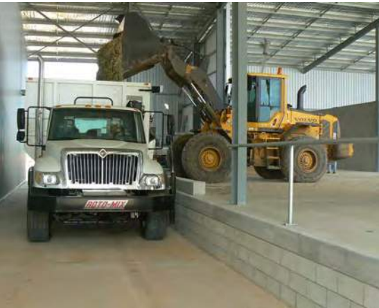
The vehicle loading area is stepped down (or the commodity area raised) so the loader can load the vehicle safely and easily.
