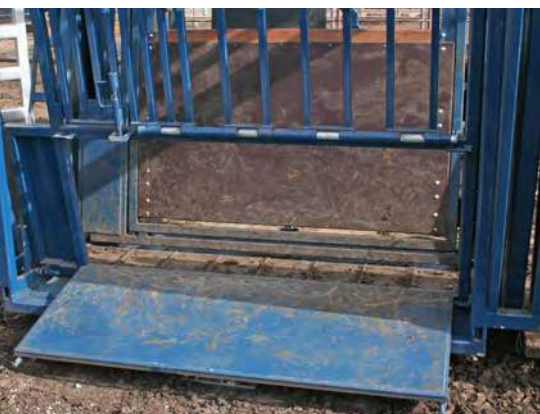
Split-side gate for release of an animal if it goes down.
