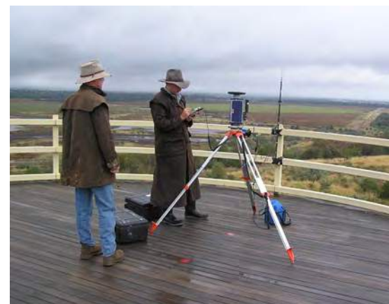
The PSM should be accessible by GPS and able to have tripod mounted above it.
