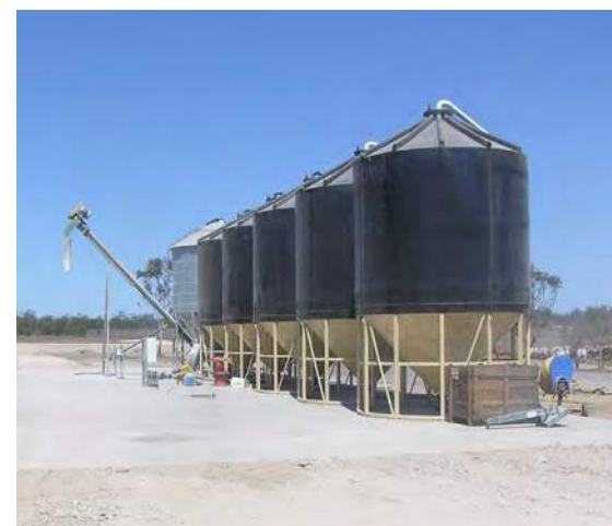
An arrangement of cone-bottom silos with a mobile auger for filling.
