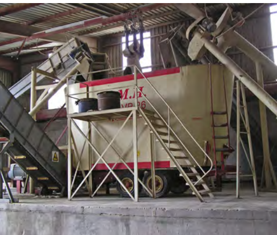
A tractor drawn horizontal vertical screw mixer set up as a stationary unit.
