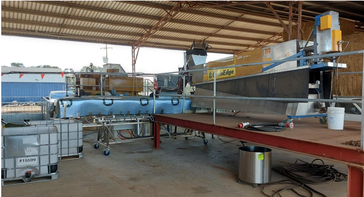
Figure 4. Setup of the GRAIN EDGE® machine for the grain devitalisation trials
