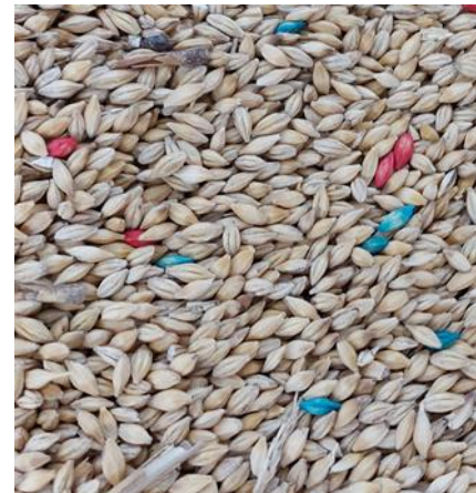
Figure 6. Dyed grain was used to determine retention time in the treatment chamber
