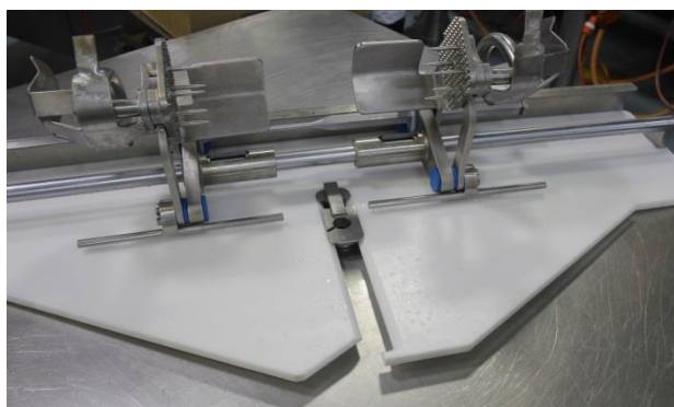
Figure 2: OP Rib attachment aligned with the bandsaw blade
