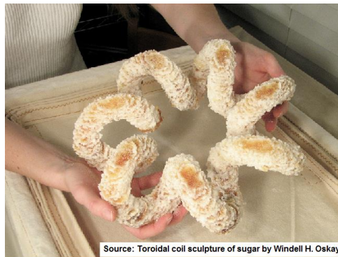
Figure 11: Example of 3D printing technique based on SHASAM technology. Image reproduced with permission from Windell H. Oskay, www.evilmadscientist.com .
