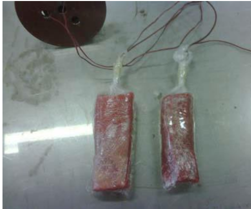
Figure 4: Sample preparation and positioning of thermocouples for temperature profiling in the 3L HPP unit.
