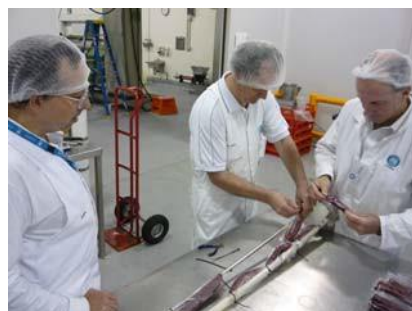
Figure 3: Method of attachment of the meat sample to the insulated sample basket for HPP treatment in the 35L unit.
