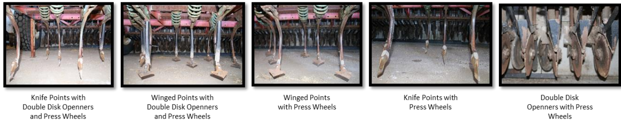
Diagram 1. Photographs of each seeding set up used underneath the International Combine
