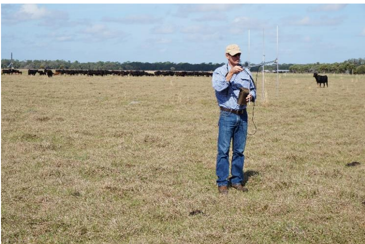
Photo 10. Tim Schatz using a portable yagi antenna to find a VHF tracking tag in Florida.
