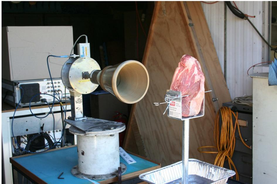
**Figure 7.** Photograph of the measurement setup showing the X-band horn, sample holder and “Beef” sample.
