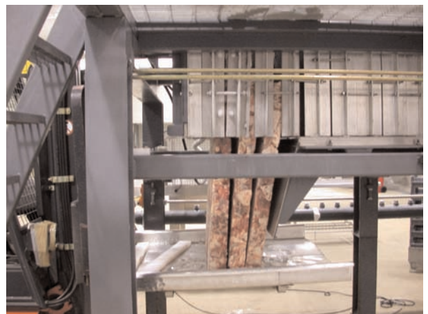
Figure 1: Unloading frozen blocks from the plate freezer
