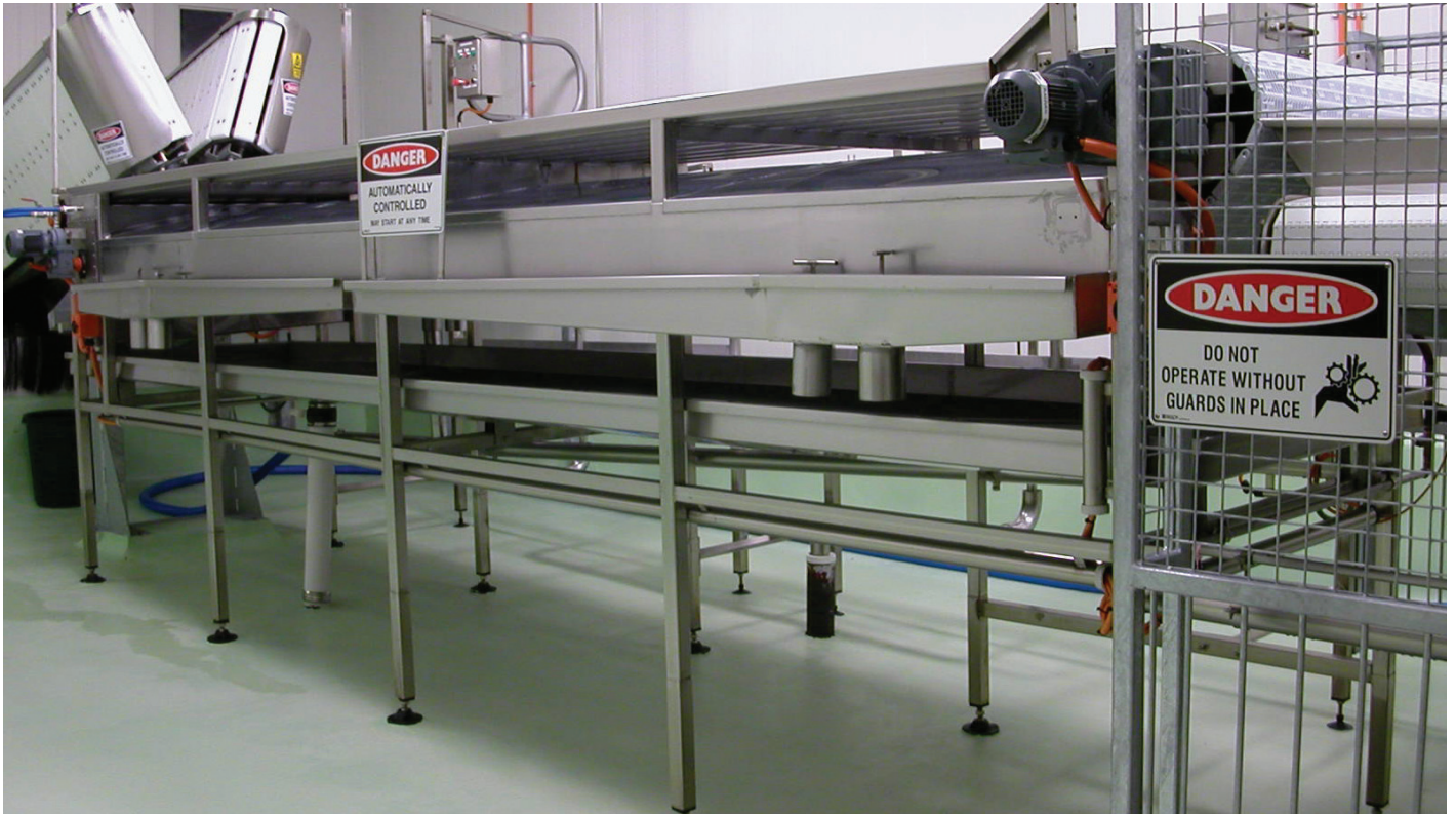
Figure 1: Modified restrainer and bleed table installed with automated dehairer
