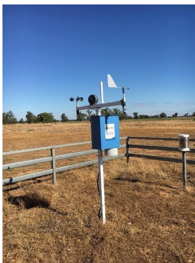
Figure 15 Weatherman AWS linked via mobile network (4G tower in ~ 10 km away)
