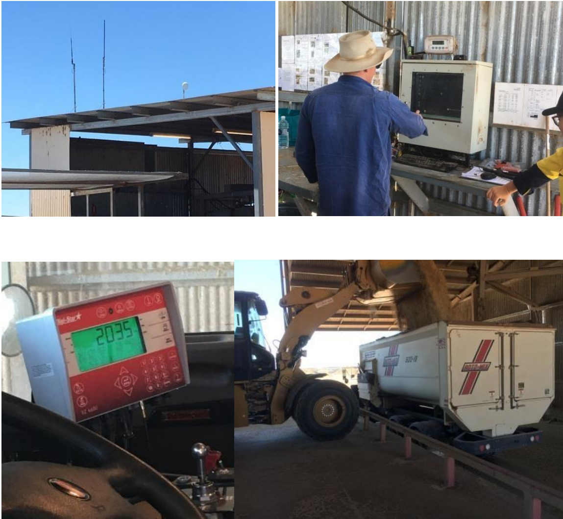
Figure 11 DigiStar operating between the Mill and Feed vehicles is facilitated by radio link direct to the Mill and Livestock section.
