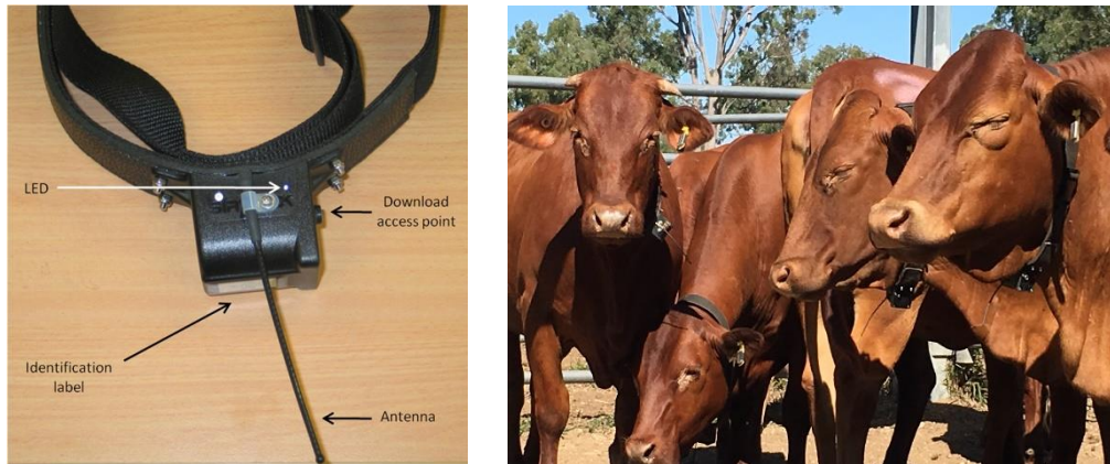
Figure 1. Left: The external components of a proximity logger collar, Right: cattle fitted with proximity logging collars
