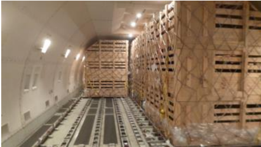
Appendix B20: Positioning of triple tiered crates into the main hold.
