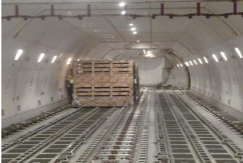
Appendix B19: Positioning of a double tiered crate within the main hold.
