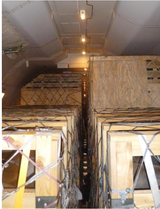
Appendix B4: Layout of single and double tiered crates. Note the space between crates down the centre of the hold. This area was identified as “Hot Spots”, where air flow and therefore heat flux would be lower.
