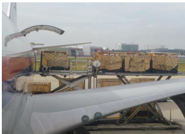
Appendix B16: Loading of single tiered crates through the main hold cargo door at the aft of the aircraft.
