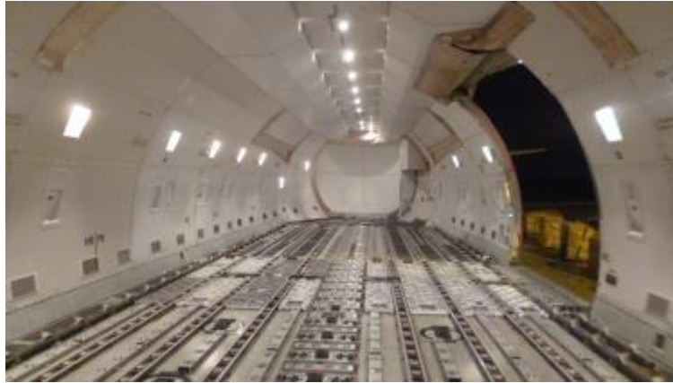
Appendix B17: View of the aft of the main hold showing cargo door access.
