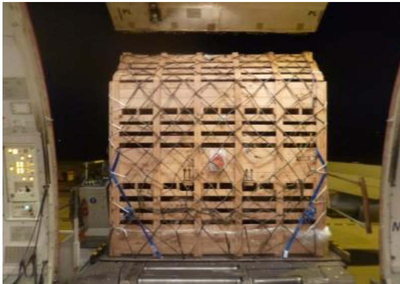
Appendix B18: Loading of a triple tiered crate through the cargo door of the main hold.
