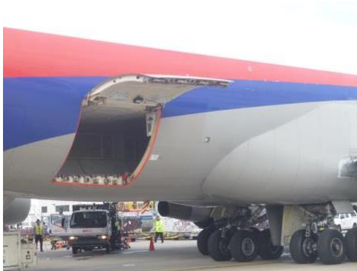
Appendix B15: Bottom aft hold cargo door opened for loading of single tiered crates.
