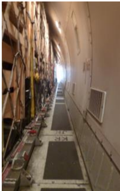
Appendix B5: Distance between crates and fuselage wall of the main hold. Exhaust vents run down the hold near the floor.
