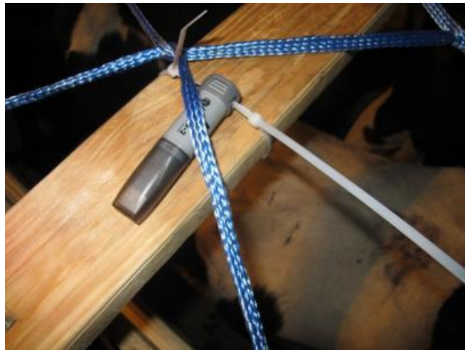
Appendix B1: Temperature and humidity logger attached to the roof of a single tiered crate.
