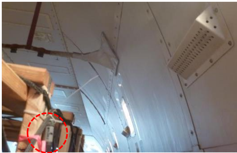
Appendix B2: Ventilation shaft next to a single tiered crate with a temperature and humidity logger attached.
