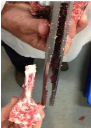
Figure 24: Blades cut either side of spinous process include a stepped gap
