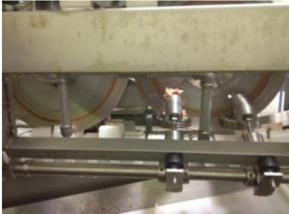
Figure 28: Two circular knife blades offset from each other cut through either side of the chine bone
