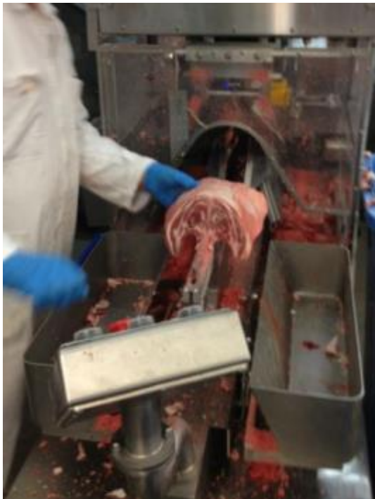
Figure 14: Carriage enters chining saws after operator positions rack and presses button on console. Carriage retracts with chinned racks in trays. Operator removes racks to belt or table.
