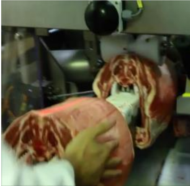
Figure 12: Manual loading of rack onto loading conveyor with laser centring guide. Manual button above rack indexes chain forward when pressed. Roller holds rack in position.
