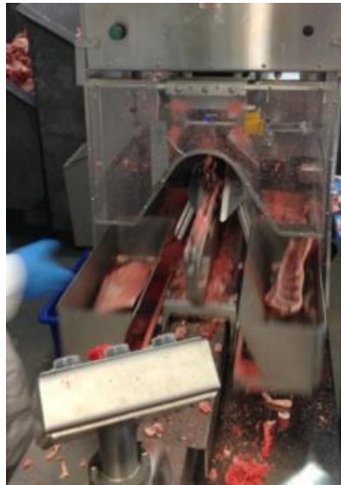
Figure 14: Carriage enters chining saws after operator positions rack and presses button on console. Carriage retracts with chinned racks in trays. Operator removes racks to belt or table.
