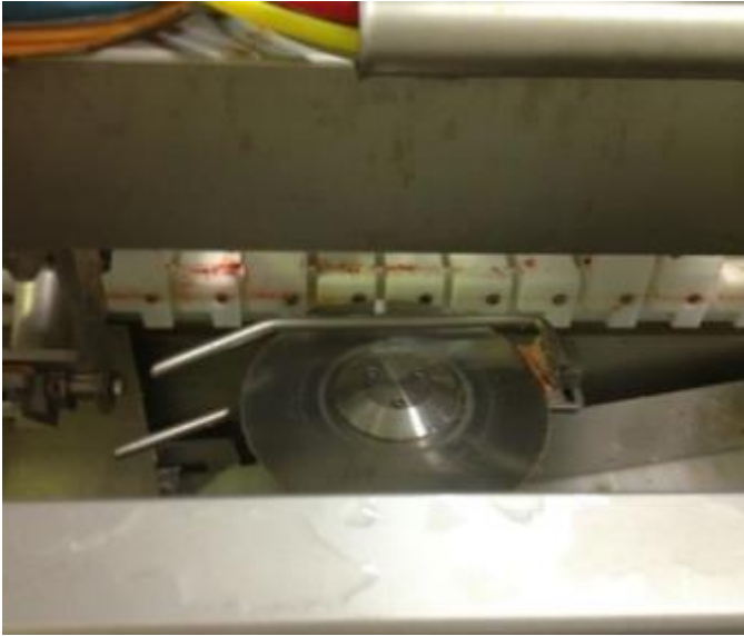
Figure 38: Flap removal saw on either side of conveyor cut adjustable flap lengths
