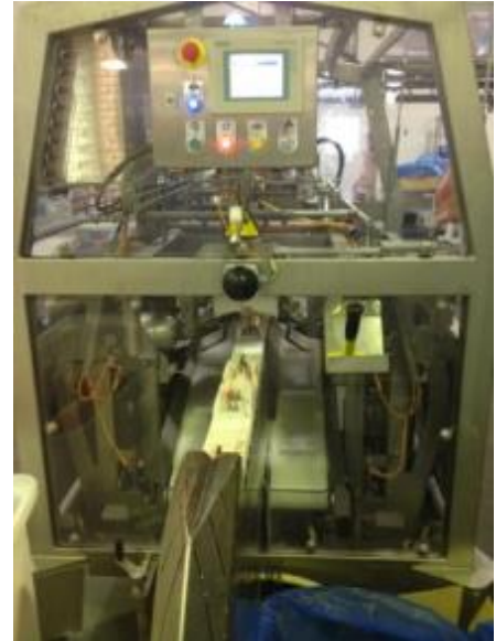
Figure 39: Continuous in-feed conveyor length customised to site requirements. Digital controls change flap length in-line.
