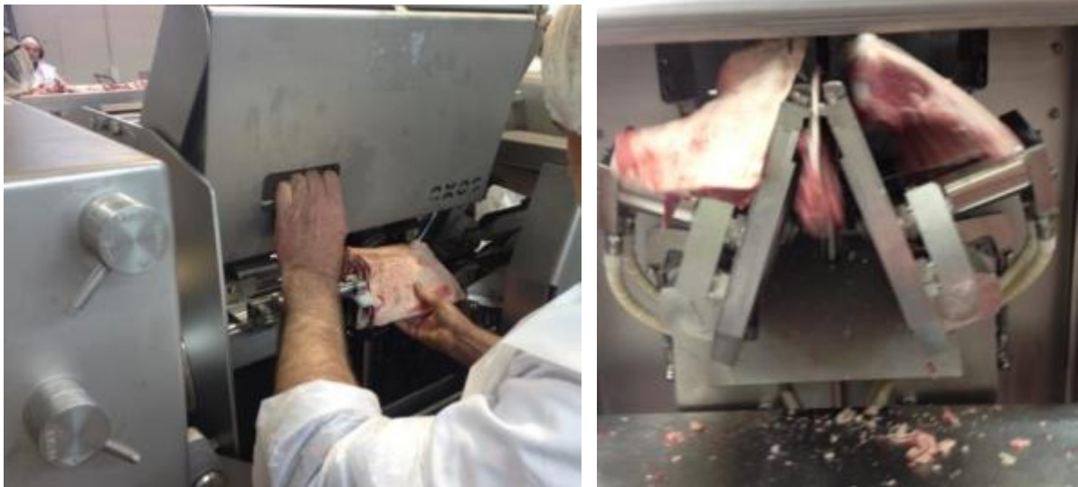
Figure 15: Operator loads rack in chamber. As door is closed holding mechanism grasps rack then pushes rack through knife and saws. Chine bone and racks exit machine onto belt or table
