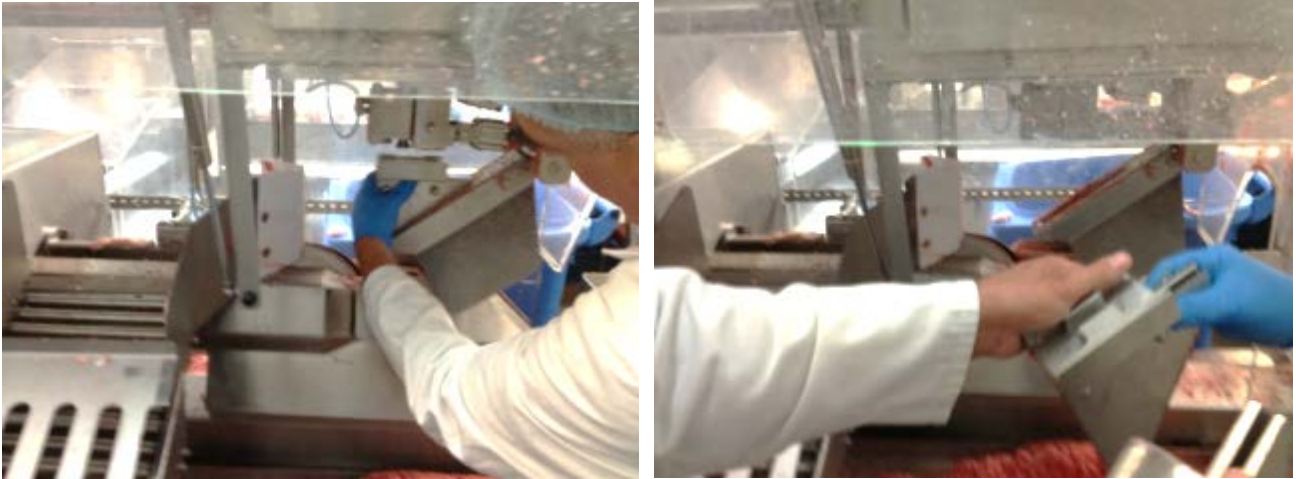
Figure 26: Removal of the blade mechanism for sharpening and adjustment is an easy quick release process
