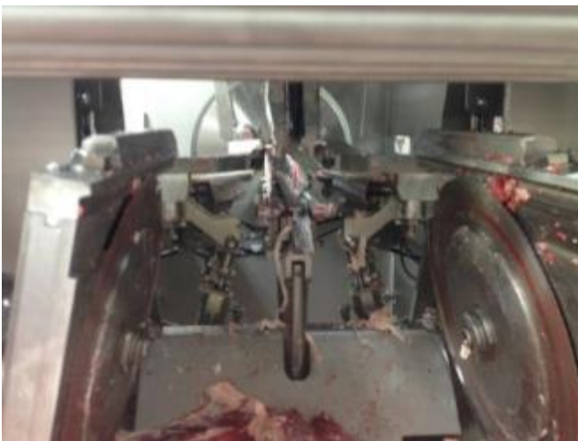
Figure 40: Loin mode (chine saws move out of the cutting path)
