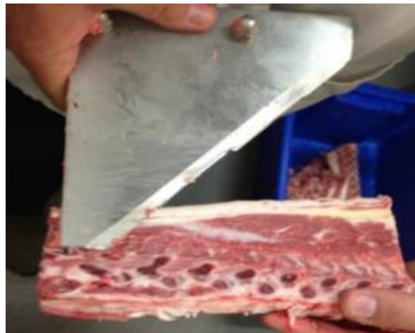
Figure 25: Demonstrates the way the chine bone passes between the blades while separating from the loin muscle on the rack. The stepped gap allows the thicker tip of the vertebrae to fit through while still cutting close to the narrow portion of the spinous process
