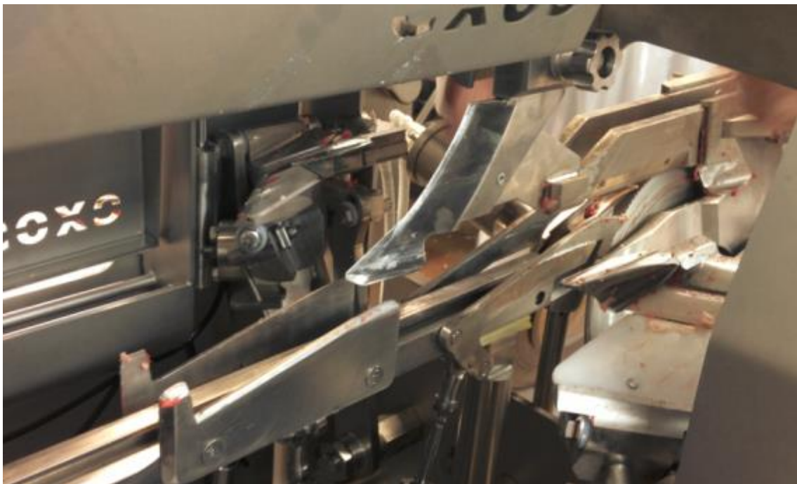
Figure 31: Macpro knife mechanism separates muscle from vertebrae above ribs, followed by saw removing rib as a second cut in the foreground of Figure 30
