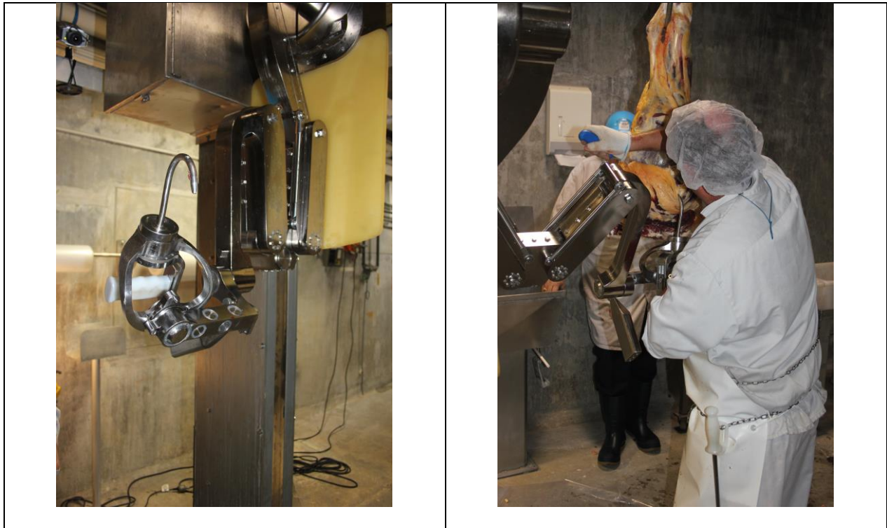
HookAssist installed and being trial in a chiller at NCMC.
