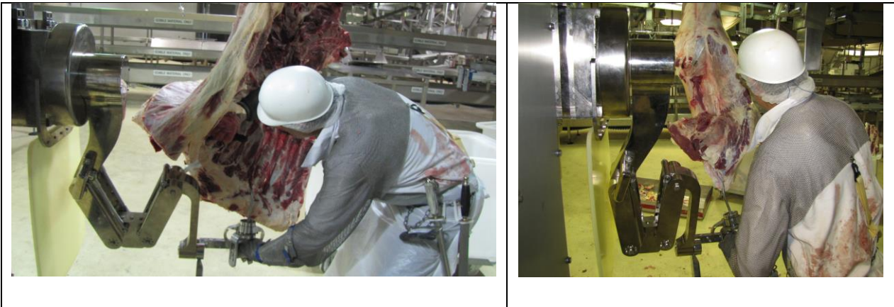
HookAssist installed in 'spare' boning room at Brooklyn
