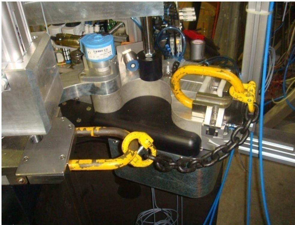
Figure 34: Shackle Links Successfully Loaded into the Beef Shackling Tool
