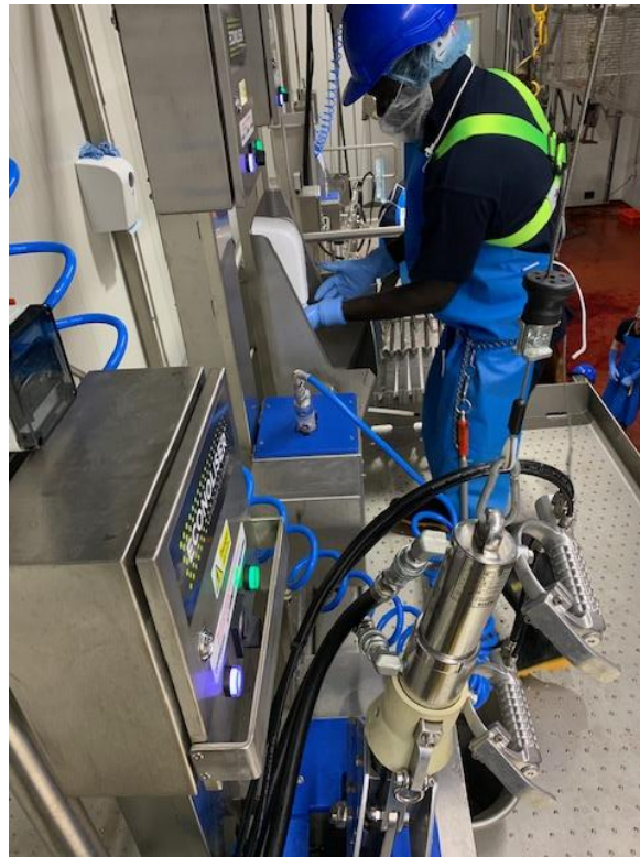
Figure 4: Operation of a 1st leg hock cutter steriliser and air knife steriliser
