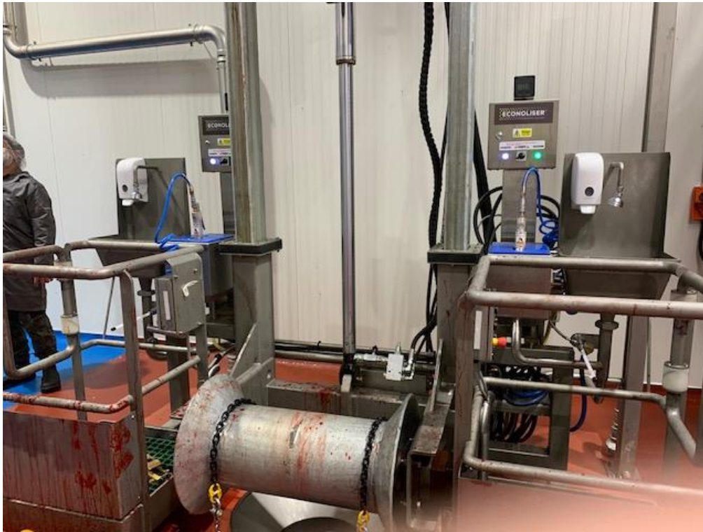
Figure 6: Operation of a dual steriliser for air knife and conventional knife on hide puller
